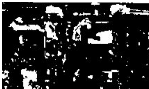
Figure 4: A change mask produced by performing Simple Differencing algorithm on images from Figure 3.
