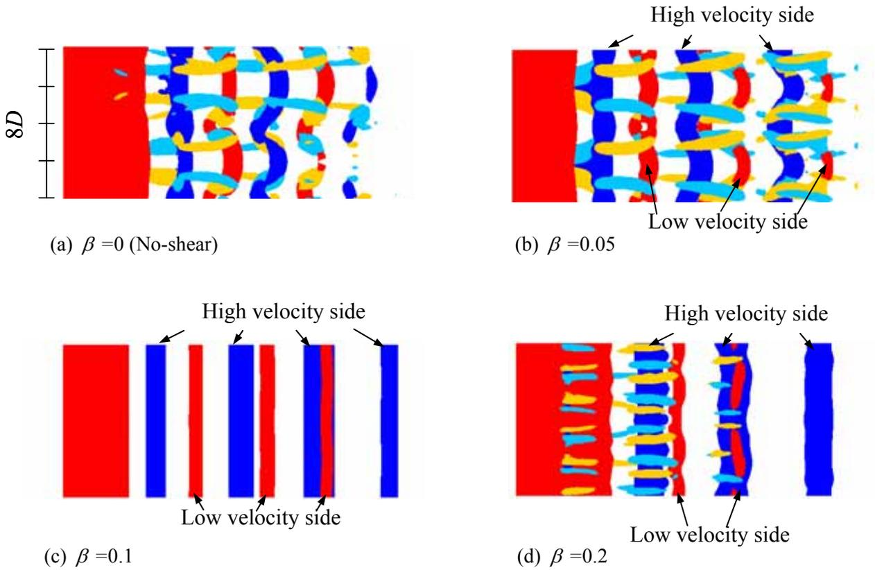
Fig.3 Variation of iso-vorticity surface of instantaneous wake structure with shear parameter at  $Re=200$
