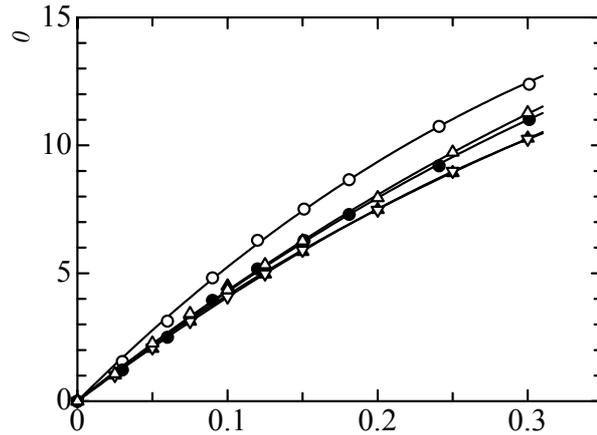
Fig.4 Movement of stagnation point with shear parameter
