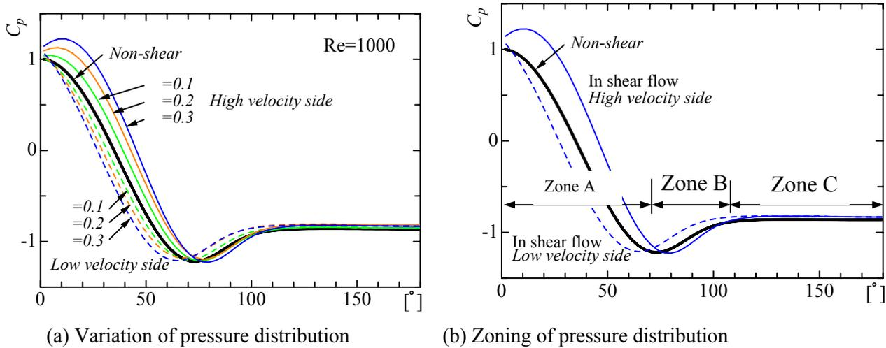
Fig.8 Variation of pressure distribution with shear parameter and its zoning
