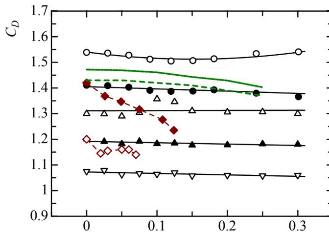
Fig.9 Variation of drag coefficient with shear parameter at different Reynolds numbers
