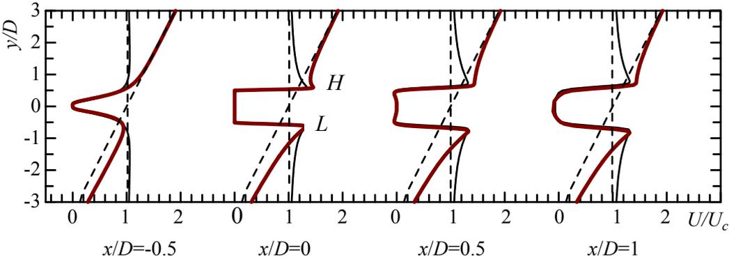
Fig.6 Mean velocity field around the cylinder ( $Re=1000, \beta = 0.2$ )
