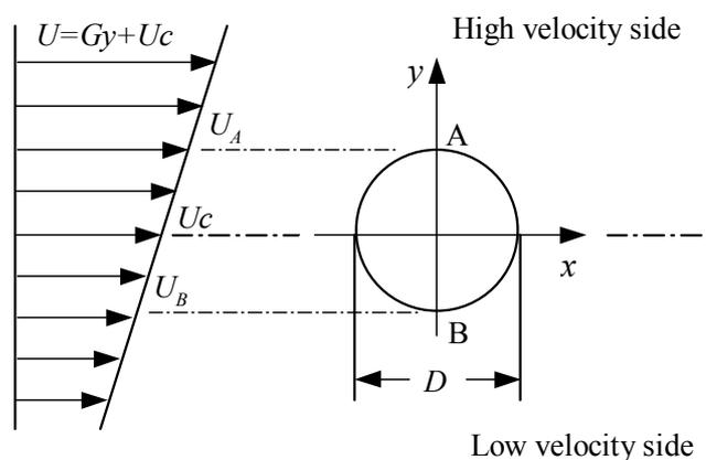
Fig.1. Schematic of shear flow configuration
