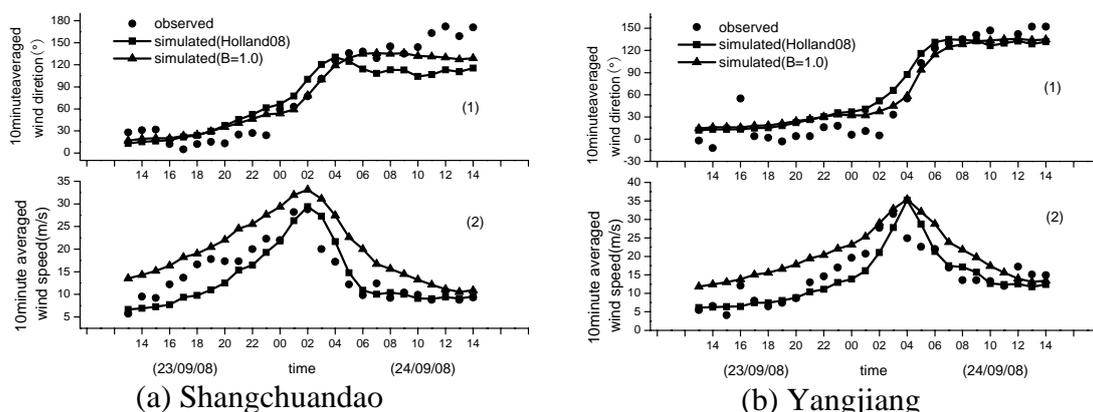
Figure 2: Comparison of Observed and Simulated Wind Speeds of Typhoon Hagupit with  $B$  Determined by Holland08 and  $B$  set as one
