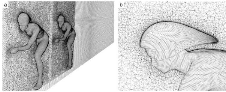
Figure 2: (a) Grid for two drafting cyclists in time-trial position and with bicycle separation distance  $d = 0.01$  m. (b) Detailed view of computational grid near upper body, head and helmet.
