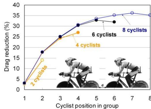
Figure 3. Numerically simulated drag reduction in groups of 2, 4, 6 and 8 cyclists, in time-trial position with bicycle separation distance  $d = 0.01$  m.
