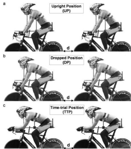
Figure 1: Three cycling positions with indication of bicycle separation distance  $d$  (wheel-to-wheel): (a) Upright position (UP); (b) Dropped position (DP) with straight arms; (c) Time-trial position (TTP).
