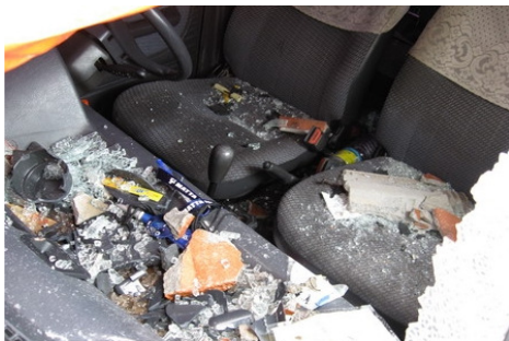
Figure 4c: Damage Due Flying Debris
