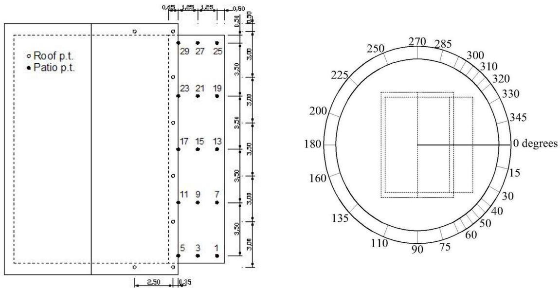
Figure 9. Pressure tap location and notation on the patio cover model and examined wind directions.
