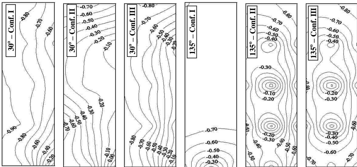
Figure 10. Correlation coefficient contour plots for top and bottom pressure signals (30 and 135 degrees wind direction).
