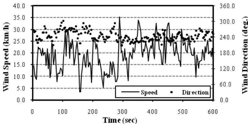
Figure 6. Typical wind speed and direction records.
