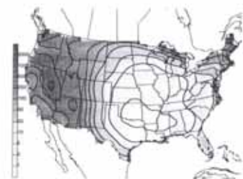
Figure 10: Return period for F2 or greater tornadoes in thousands of years from Monte Carlo simulation. Note that contours follow progression 1, 2, 5, 10, etc.
