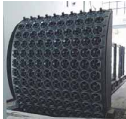
JT-6 (B1.5m × H1.8m × L10m) (12 × 10 individually-controlled fans)
